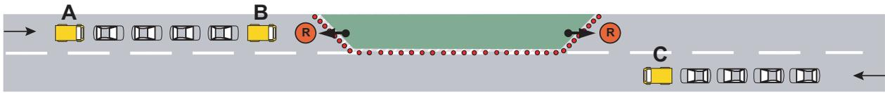
1. Initially the signs at both ends are on "STOP". The convoy escort vehicles are labelled A, B and C.
